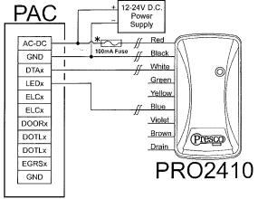
**Note** that the Green, Yellow, Violet, Brown and Drain wires are not connected when the PRO2410 is used with a PAC decoder.
