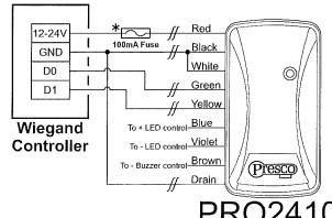
**Note** that the White wire is connected to GND (Black wire) at the PRO2410, but the Drain is connected to GND at the Wiegand controller.
